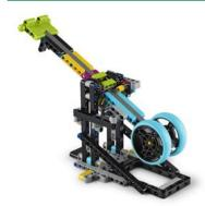
Before the match, you hand select the machine's lever setting. During the match, the robot moves the lever until the little yellow stopper falls.
