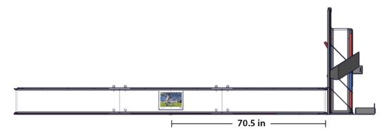
• The Navigation Image horizontal center line should measure 6.375 inches to the floor (5.75 inches from the top of the tile).
