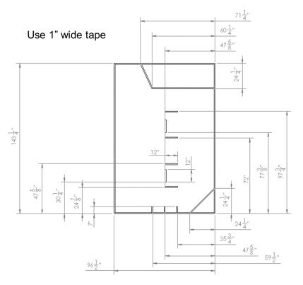
C-14 Dimensions of taped field (red side shown)
