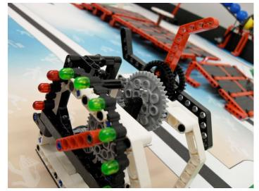
**WEIGHT MACHINE** – Dual Lock in 8 places as shown in the picture. Omit the pairs indicated by the rings. Set position is with the wheel hanging directly down, and with the ratchet/catch lever resting on the east side as shown.
