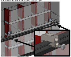
**Step 1-14:** Locate two Beam Clamp Assemblies and loosen the screws enough to fit over the field perimeter.
