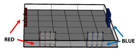
**Step 1-12:** Place two Lower Clips around the bottom of the field perimeter rail with the longer tab on the inside of the perimeter. The clips will secure the center two extrusions on the Cryptobox to the perimeter.
