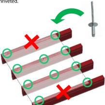
**Step 1-5:** Ensure that the Back Panel is aligned and secure each rivet using a rivet tool. Place the pin of the rivet into the hole in the rivet tool and squeeze the handle together until you hear a snapping sound. The rivet pin will detach from the rivet and the two pieces will be secured together.
