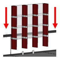
**Step 1-15:** Place a Beam Clamp on either side of the Cryptobox with the screw on the outside of the perimeter for the AndyMark perimeter. For IFI perimeters the screws should face downwards. Tighten the screw and nut to secure to the rail but be careful not to crush the rail.
