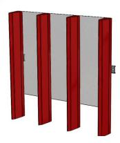
**Step 1-9:** On the back flat surface, three lines of 1" white gaffers tape should be added. The bottom edge of the tape should sit at 6, 12, and 18" measured from the bottom edge. The line extends across the full width of the Cryptobox.
