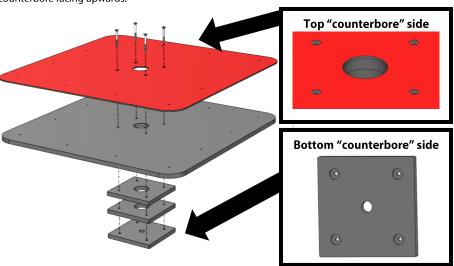
**Step 2-4:** Secure the stack together with the four 10-32 x 2.00" Screws and 10-32 Nylock nuts. Tighten until the heads of the screws are flat with the surface of the RED or BLUE panel and the nuts are flush with the inner bore of the bottom panel. Bolts may need to be temporarily loosened for step 2-5.
