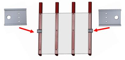
**Step 1-7:** Using rivets, secure each Cable Tie Bracket to the extrusions. Use three rivets per bracket.
