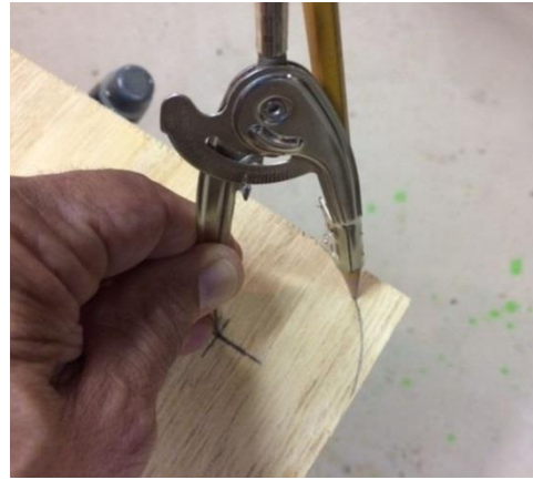
Figure 9: Use a compass to trace a quarter circle on each corner.
