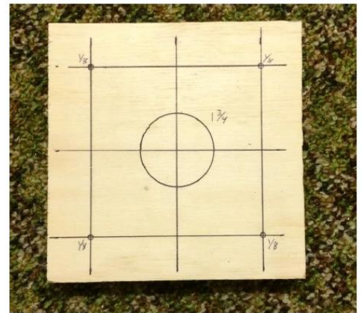
Figure 13: Measure holes for the Balancing Stone - Upper Pylon
