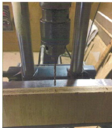
Figure 3: Drill 24 holes (6 per rail) in Main Rails
