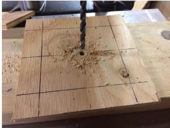
Figure 30: Drill the 1/4" diameter center hole with a 1/4" drill bit.
