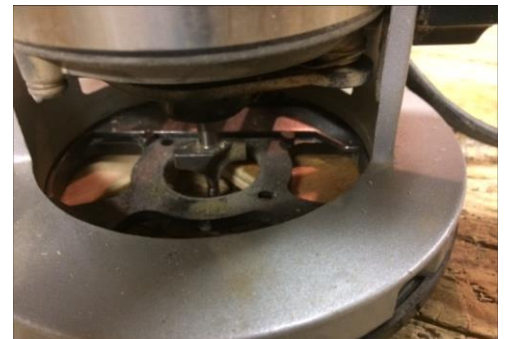
Figure 5: You can also use a 45 degree router bit and a router to chamfer the edge of the wood.
