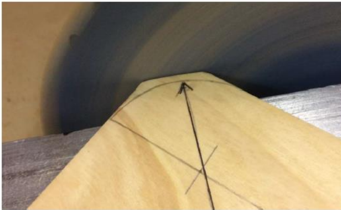
Figure 10: Sand rounded corners down to a 2" (5.08cm) Radius.
