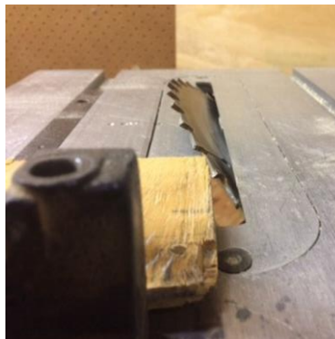
Figure 22: Set table saw to 45 degree angle.
