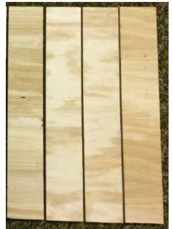
Figure 2: Cryptobox Main Rails (4 in total) - 4"x24" (10.16cm x 60.96cm)
