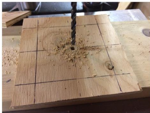
Figure 27: Use a 1/4" Drill Bit to drill the center hole in the Balancing Stone - Lower Pylon.
