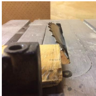
Figure 5: Set table saw to 45 degree angle.
