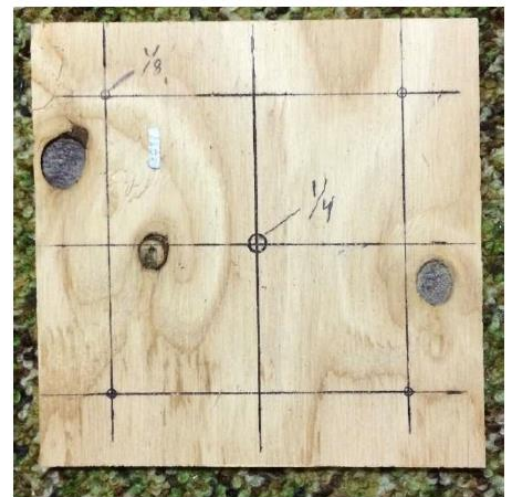
Figure 25: Measure, cut and draw drill holes for the Balancing Stone - Lower Pylon.
