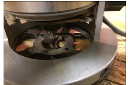
Figure 23: You can also use a 45 degree router bit and a router to chamfer the edge of the wood.
