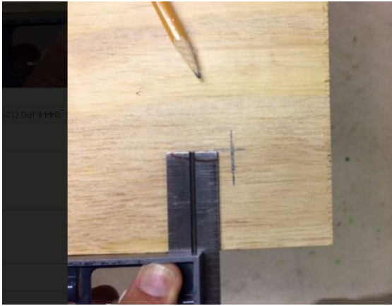
Figure 8: Measure a center point 2" (5.08cm) from each side.
