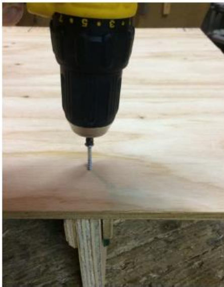
Figure 36: Drill from the back of the Cryptobox Back Panel.
