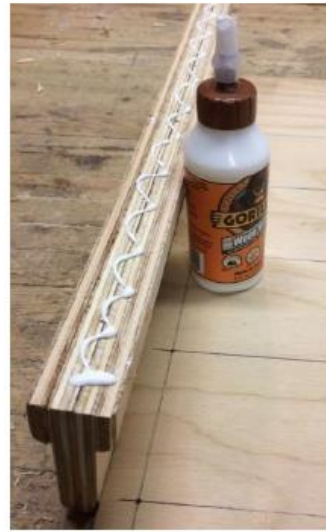
Figure 35: Apply wood glue to bottom surface of Rail Assembly.
